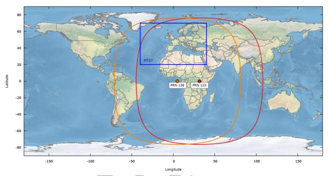
Figure 1: Coverage of EGNOS GEOs with 5° masking angle
