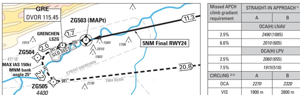
Figure 1 – Grenchen AD (Switzerland). Snapshot CTR/RMZ – OCA(H)
