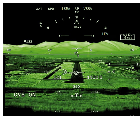
Head Up Display while flying an LPV approach at night with FalconEye combined vision system (CVS) Credits: Dassault Aviation
