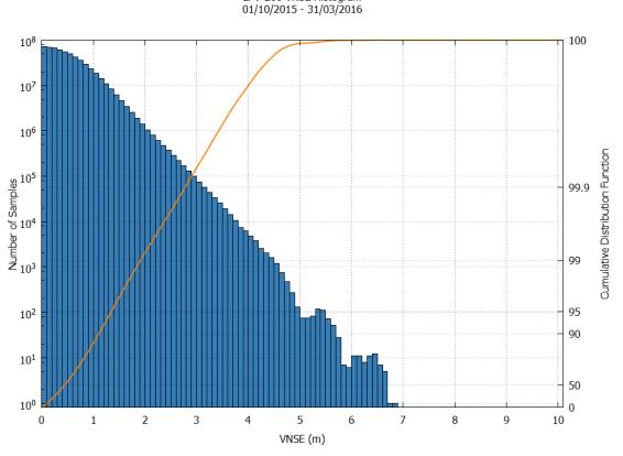
Figure 33: EGNOS LPV-200 Vertical Accuracy Histogram and Cumulative Probability
