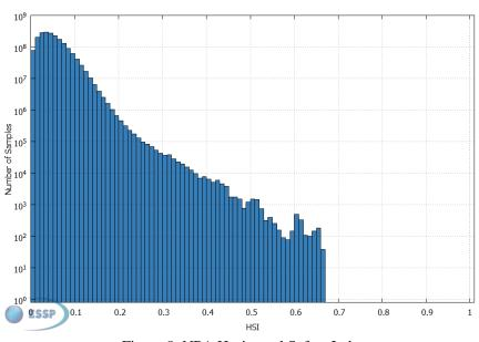
Figure 8: NPA Horizontal Safety Index
