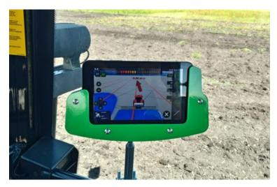
Steering system installed on a tractor
