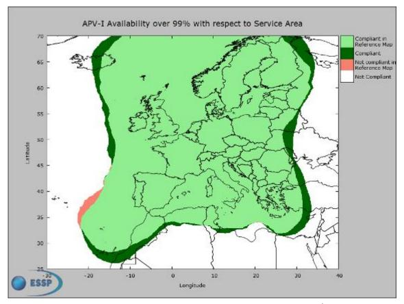
Figure 12: APV-I 99% Availability map with respect to the 99% APV-I Service Area<sup>4</sup> - 01/04/17 to 31/03/18
