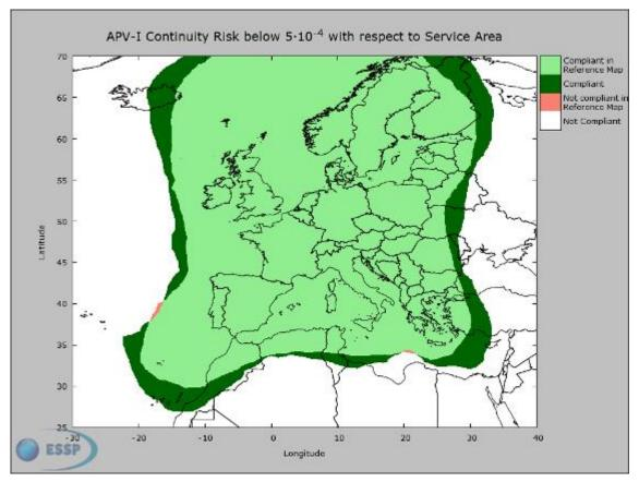
Figure 18: APV-I Continuity Risk  $(5 \cdot 10^{-4})$  map with respect to the  $5 \cdot 10^{-4}$  APV-I Service Area<sup>7</sup> - 01/04/17 to 31/03/18
