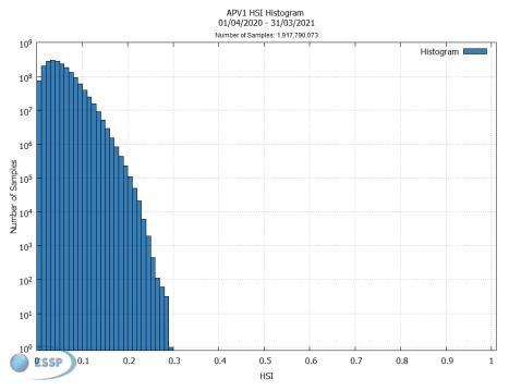
Figure 13: EGNOS APV-I Horizontal Safety Index<sup>6</sup>
