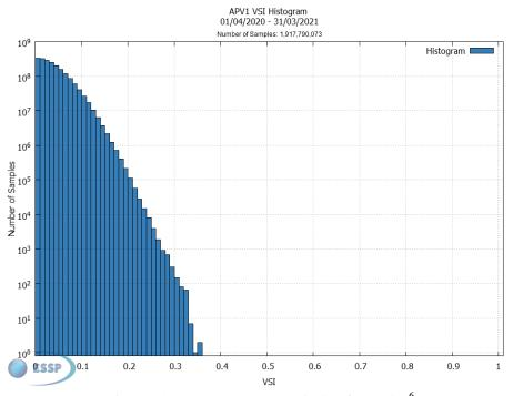
Figure 14: EGNOS APV-I Vertical Safety Index<sup>6</sup>
