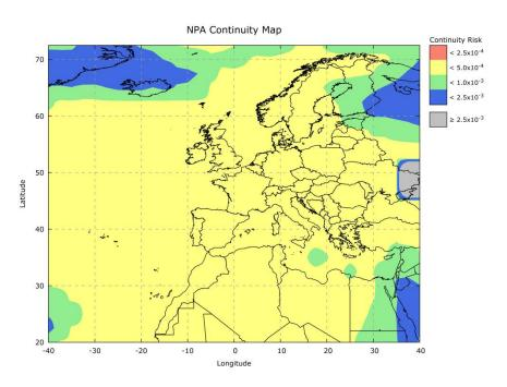
Figure 3: NPA Continuity map - Expected minimum performance (SoL SDD v3.3)
