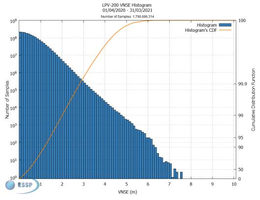
Figure 26: EGNOS LPV-200 Vertical Accuracy Histogram and Cumulative Probability
