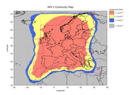
Figure 9: APV-I Continuity map - Expected minimum performance (SoL SDD v3.3)
