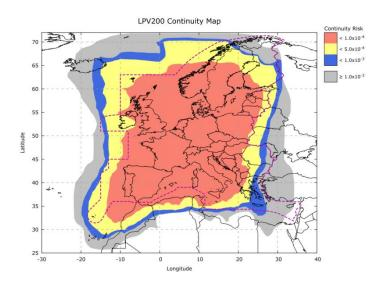
Figure 18: LPV200 Continuity map - Expected minimum performance (SoL SDD v3.3)
