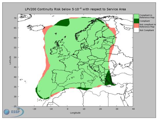
Figure 25: LPV-200 Continuity Risk  $(5 \cdot 10^{-4})$  map with respect to the reference map - 01/04/20 to 31/03/21 In the picture, the legend should be read as follows:
