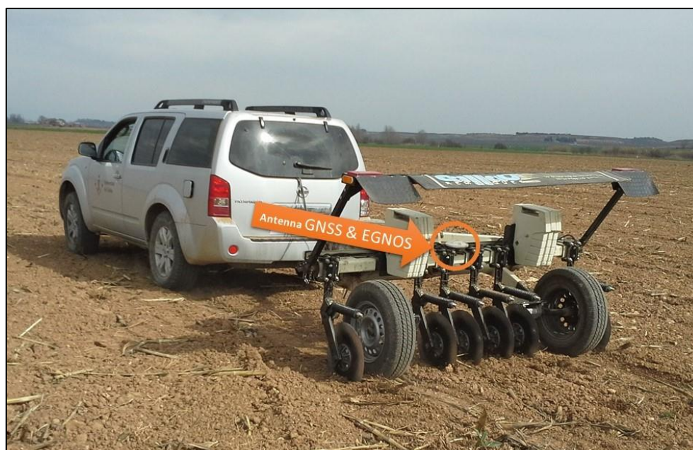
Figure 38: The University of Lleida measures soil ECa using a device that georeference the measurements using EGNOS (credits: University of Lleida)
